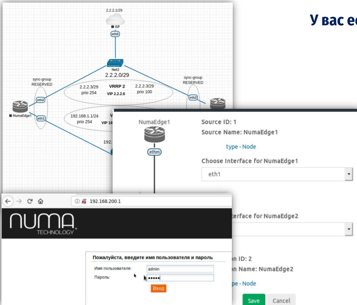
The image displays a network diagram and the Numa Edge configuration interface. The network diagram shows a central router (Net2) connected to an ISP (2.2.2.1/29) and two edge routers (NumaEdge1 and NumaEdge2). The central router has a VRRP 2 configuration with VIP 2.2.2.6. The edge routers have interfaces eth1 and eth2. The configuration interface shows the configuration for NumaEdge1, including Source ID, Source Name, and interface selection (eth1).
